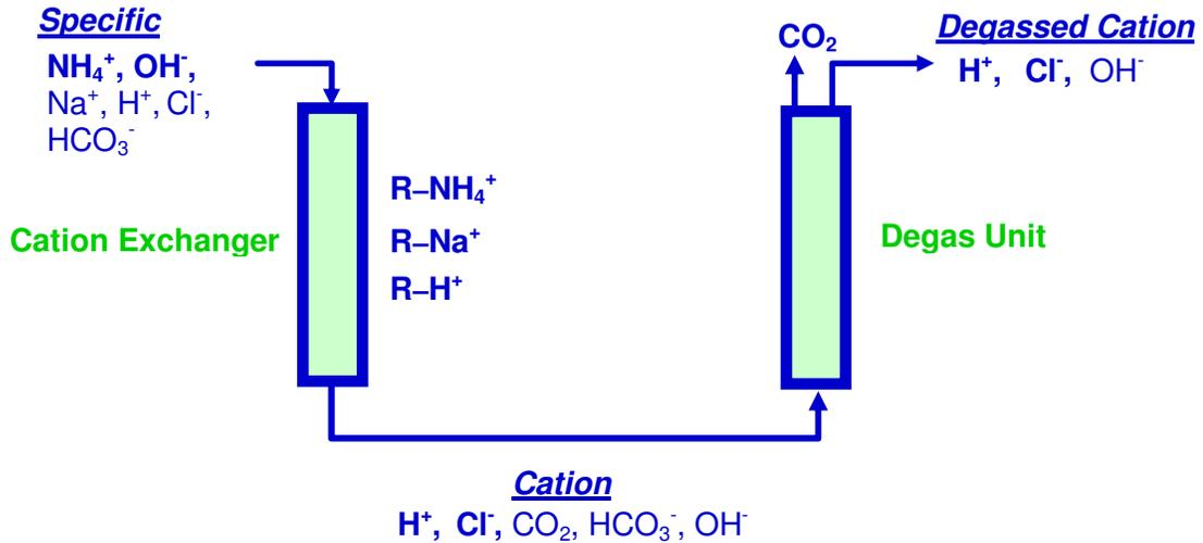
Figure 5 - Specific, Cation and Degassed Cation Conductivity Measurements
