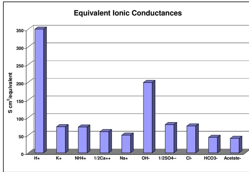
Figure 1 - Conductance of Common Ions at 25 °C
