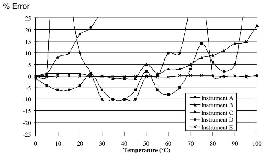
Figure 8 - Cation Conductivity Temperature Compensation Performance at 0.1  $\mu\text{S}/\text{cm}$
